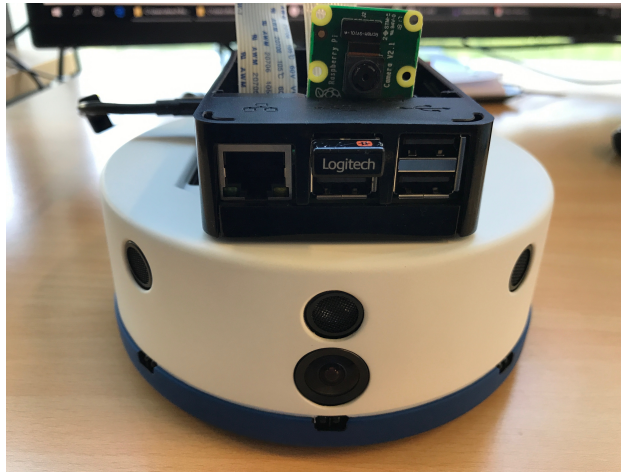
Figure 3. Khepera IV mobile robot with Raspberry Pi 3 and camera on top.
